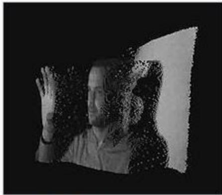
Range image of a human face captured with a time-of-flight camera (artist's depiction)
