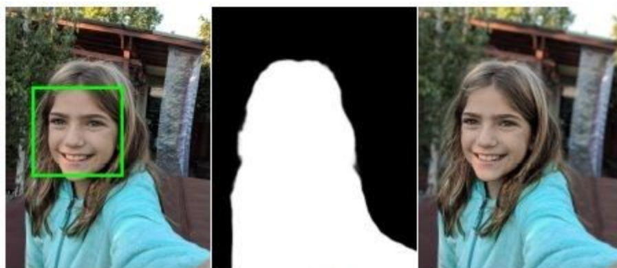
Input Mask Output (a) A segmentation mask obtained from the front-facing camera.
